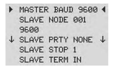
The MGS-408 controller acts as a MODBUS master device on the detector side, and as a MODBUS slave device on the BMS side.
