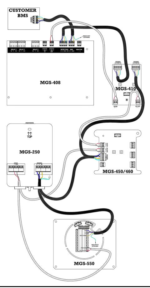
Locate the RS-485 connectors in the MGS-408 Gas Detection Controller. The left RS-485 connector is for downstream "slave" devices (includes a dedicated shield position) and the right RS-485 connector is used to connect to "master" devices upline, such as building management controls.
